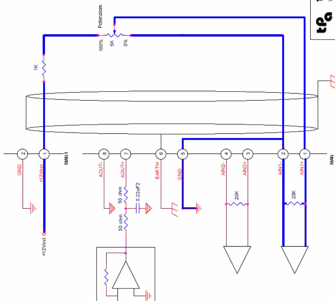
Any metal box of the potentiometer must be adjusted at zero potential.
